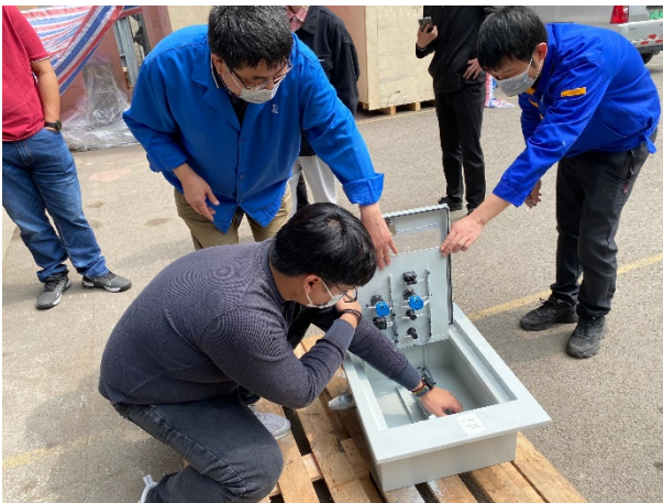
HANDS ON LEARNING... Engineers and technicians are conducting a thorough inspection of a local control panel following the completion of a dust resistance test.
